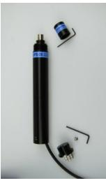
Lift off the adjustment tool and insert the adapter and mic in the OPS35 body. The microphone is installed in the correct position now.
