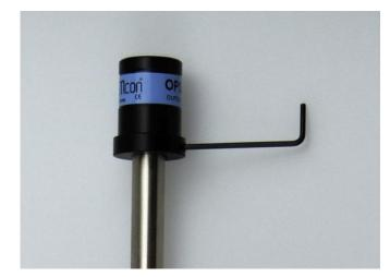
Bring the microphone adapter and the OPS adjustment tool together so the adjustment tool sits on the adapter (adapter rim slides into the cap).
