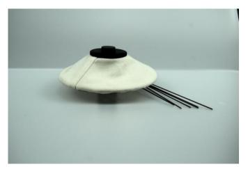
The fabric used is water tight but acoustically t ransparent as far as possible (not rubber coated). The fibers become water tight upon getting wet (ref. tent cloth). It can be removed for cleaning, replacement and/or impregnation.
