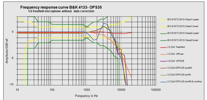
**Note**: IEC limit curves shown are for freefield equalized microphones. Additional tolerance correction for directional response will apply.
