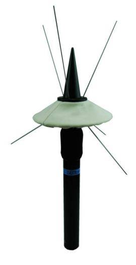
The spikes are securely installed when the bottom holder, the umbrella and weather tip are screwed together (top right picture). There is no need to add glue or epoxy.
