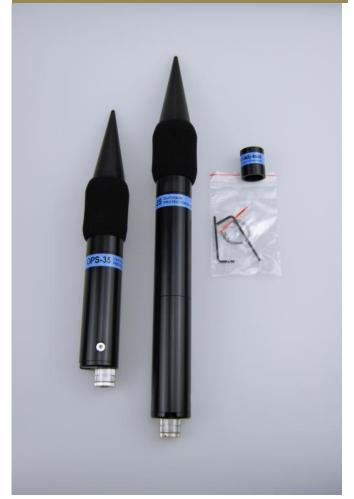
The OPS 35 system is designed to be used with a large variety of microphones in the nominal mic diameter range of 1/4" to 1/2" as well as different mic lengths.
