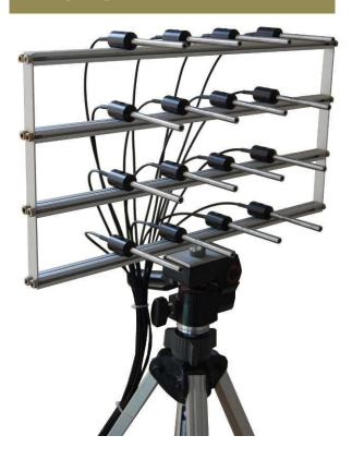
• **flexible** - built from extruded aluminum profile using pre-threaded mounting rails (1/5" spacing) or single locking nuts.
